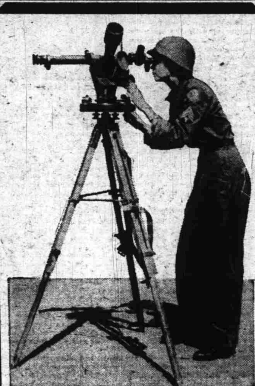
On the anti-aircraft firing range, a Wac technician operates a BC Scope, which "tracks" the low target planes and records hits and misses of Anti-aircraft Artillery soldiers.
