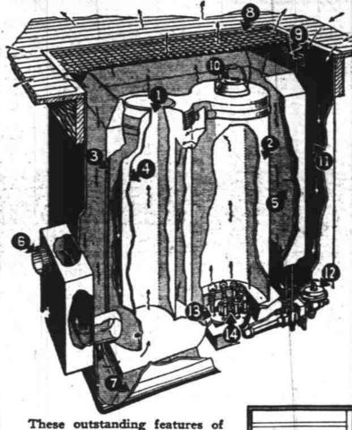
1. Streamlined Radiator and Combustion Chamber.
