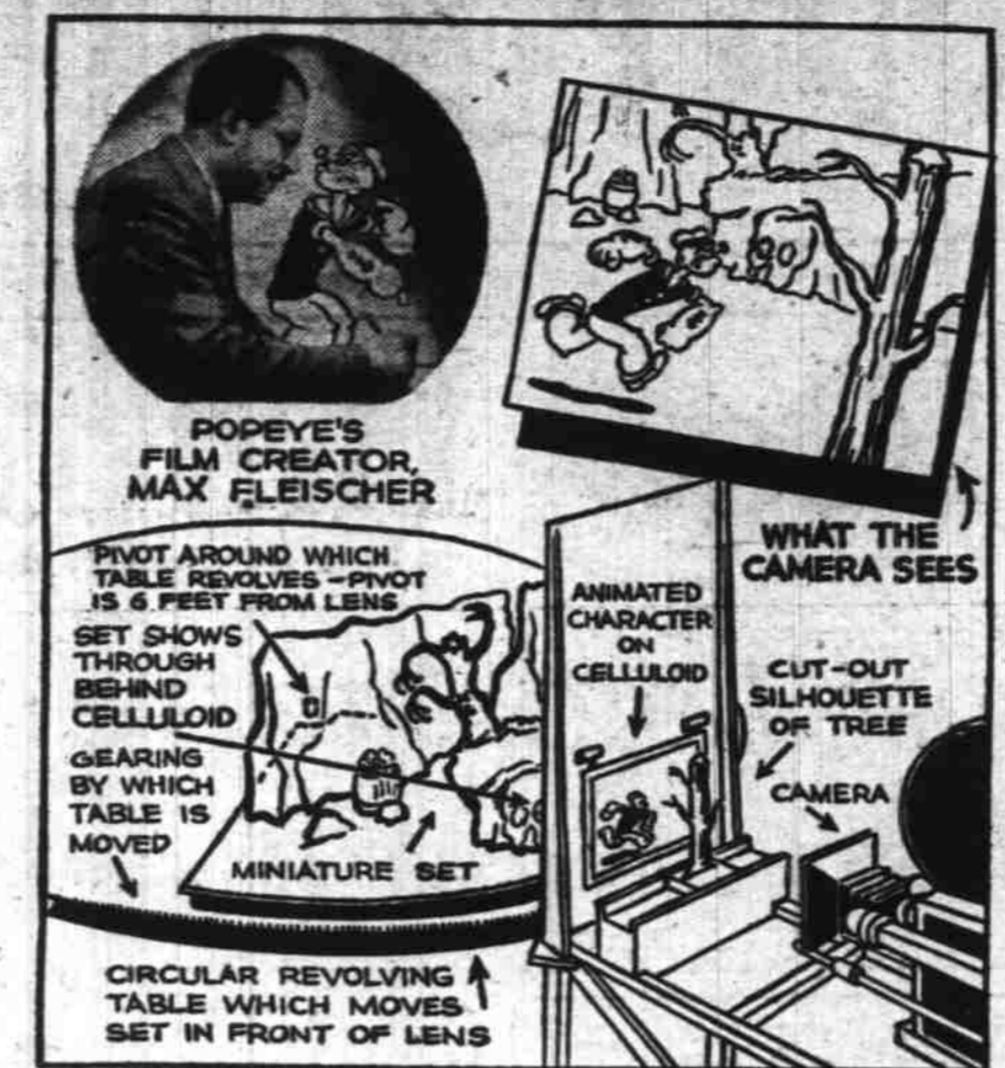
Details of the means by which Popeye gets a three-dimensional world in "Popeye the Sailor Meets Simbad the Sailor" at the State theatre Sunday are shown above.
