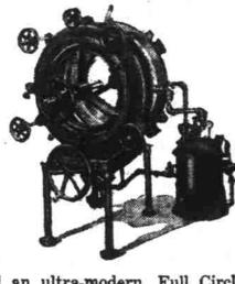
We have just installed an ultra-modern, Full Circle Retreading Mold which turns out a complete tire in one operation.
