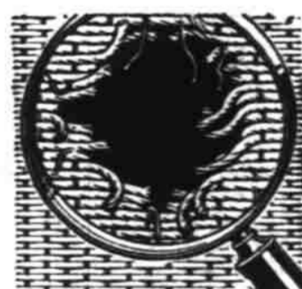
Cord Separation This shows cords that have been separated by heat inside the tire. Cord separation causes internal blistering and weakens the tire. A blowout is the result!
