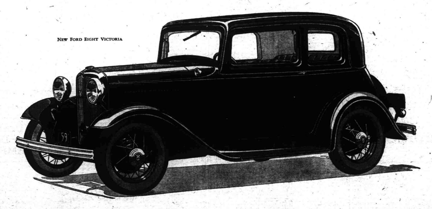
Eight-cylinder, 90-degree V-type, 65-horse-power Engine \* Vibrationless \* Roomy, Beautiful Bodies \* Low Center of Gravity Silent Second Gear \* Synchronized Silent Gear Shift \* Seventy-five Miles per Hour \* New Self-adjusting Houdaille Double-acting Hydraulic Shock Absorbers with Thermostatic Control \* Comfortable Riding Springs \* Rapid Acceleration Low Gasoline Consumption \* Reliability \* Automatic Spark Control \* Down-draft Carburetor \* Bore, 3 1/16 \* Stroke, 3 3/4
