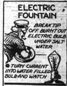
with moderately salty water and break off the top of the bulb while holding it under the water. Immediately the vacuum fountain will begin to fill the bulb with the water. When the bulb is full, put in a socket and turn on the current for a while and watch the bubbles form and rise to the top of the bulb. The water will also probably turn slightly green.
