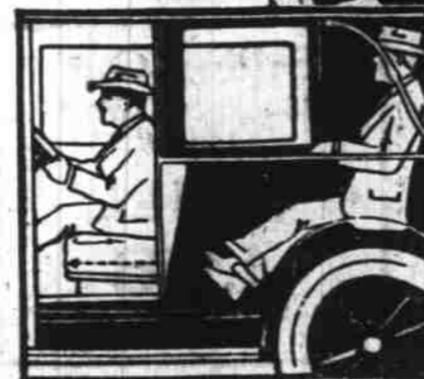
Front seat adjusts to three positions to accommodate short driver of tall driver.
