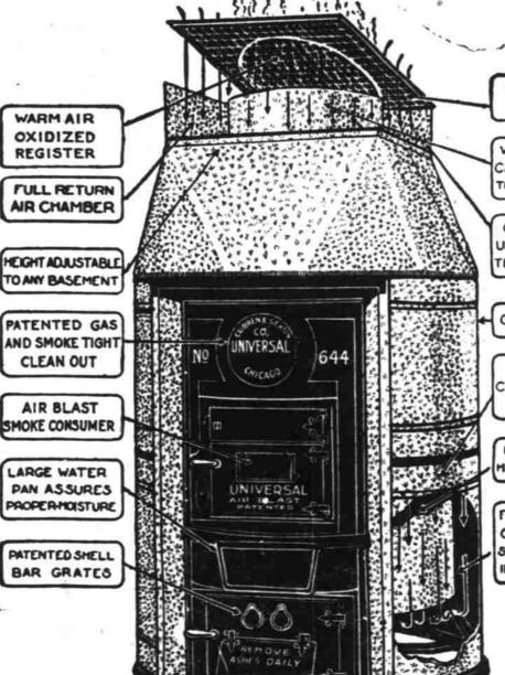
COLD AIR RETURN WARM AIR PIPE CARRIES ALL HEAT TO UPPER ROOMS COLD AIR FROM UPPER ROOMS RE-TURNS TO FURNACE
