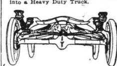
The working principle of the Olson Unit is to take the load onto the auxil-iary springs and deflect this into the steel wheels, in the housings of which
