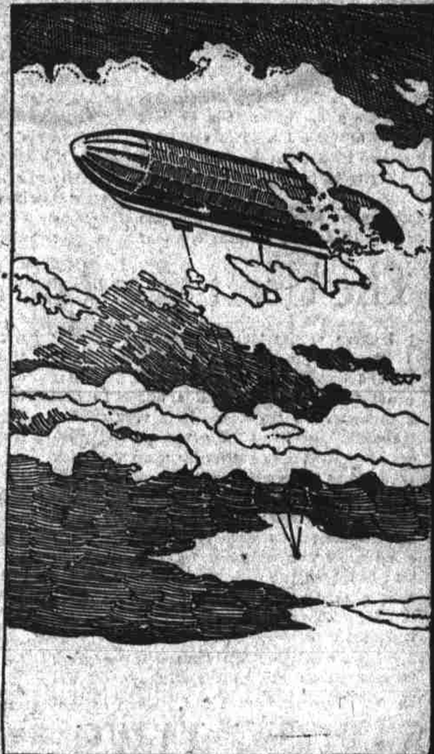
New Device Tested at Farnborough, England by Which an Airship Hidden by a Cloud Lowers a Man to Report the Enemy's Positions.
