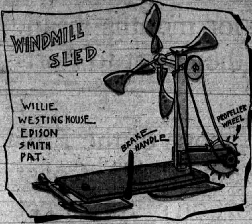
Dear Tommy—I've just built a windmill sled. I enclose a diagram so you can make one like it.
