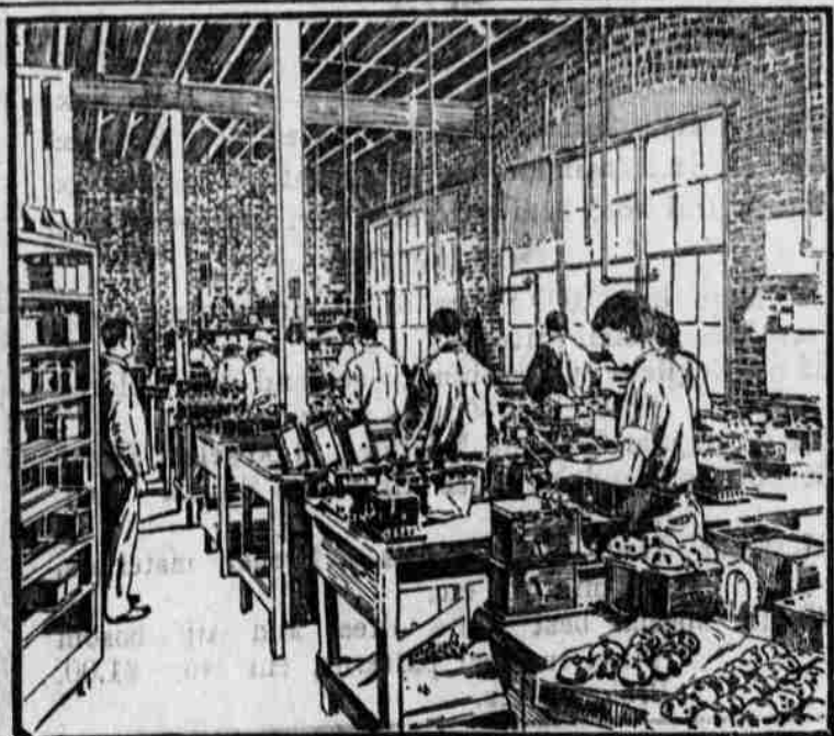
ASSEMBLING SUBSCRIBERS' TELEPHONE EQUIPMENT. The five thousand instruments produced each day in the Bell factories are made up into complete "stations" after the operating companies receive them.
