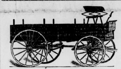
Hollow Axle, Pacific Coast Gear, with Stake Rack Bed and California Roller Brake.
