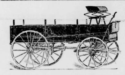
Hollow Axle, Pacific Coast Gear, with Stake Rack Bed and California Roller Brake.
