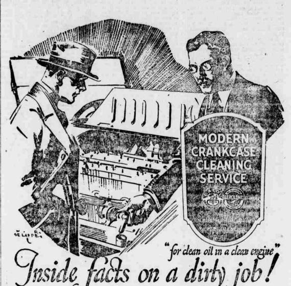
JOUR ENGINE requires an internal bath frequently. Road dust, carbon from the combustion chamber, and fine particles of metal worn from the bearing surfaces get into the lubricating oil in the crankcase. All this dirt circulates with the oil through the engine. If it isn't drained out regularly there's bound to be excessive wear and tear.
