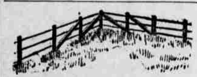
BRACING FOR THE CORNER POST.
