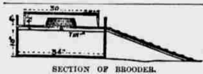
SECTION OF BROODER. and out at will, the whole being surrounded by boards four inches high and three feet long nailed together at the corners and resting on the floor of the brooder. When the chicks are ten days old one of these boards may be taken away and a bridge used so that the chicks may run from the hover to the floor of the room.
