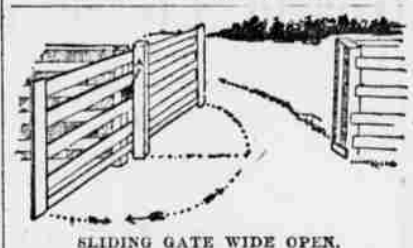
SLIDING GATE WIDE OPEN.
