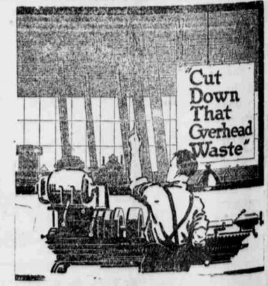
ELECTRIC DRIVE ELIMINATES LONG LINES OF OVERHEAD SHAFTING, which represents a dead loss in efficiency of as nuch as 6 per cent.
