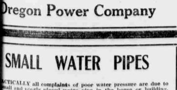
all and poorly placed water pipe in the house or building. than 2 1-2 times that flowing through 1-2-inch pipe and e cost for the larger pipe is only about 20 per cent more? have poor pressure at one faucet and good pressure at , you may be sure the house piping is at fault.
