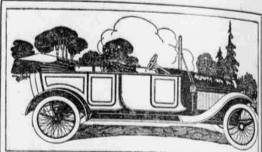
Motor-Cast en bloc, 4-cylinder, water cooled, 2% bore, 4 inch stroke, Wheelbase-102 inches.
