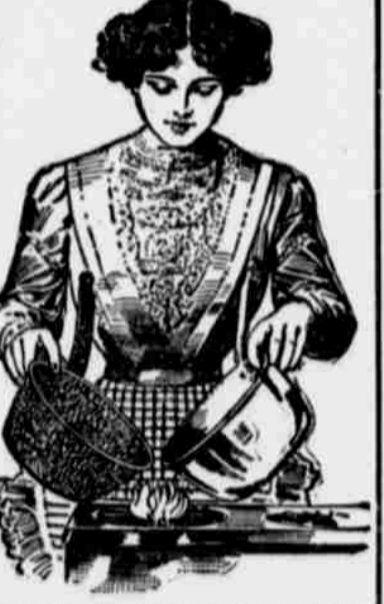
Hold by the edges an aluminum pan and an enamel pan of the same size, so that the sides opposite your hands are in a small flame, as shown in this picture. You will drop the aluminum pan first.
