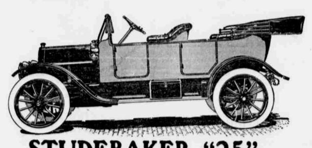
Five-passenger, Four Cylinders, Long stroke, 3 1-2-inch bore x 5-inch stroke, 102-inch wheelbase
