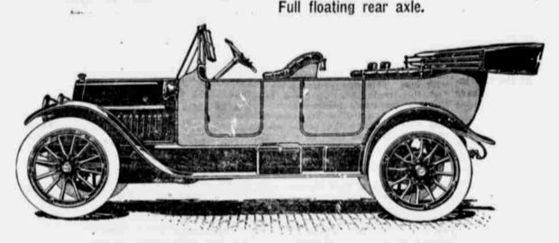
Four Cylinders, 4 1-8-inch bore x 5-inch stroke, 116-inch\_wheelbase.
