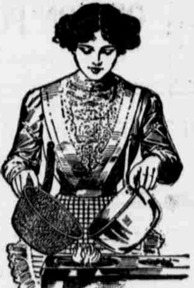
Hold by the edges an aluminum pan and an enamel pan of the same size, so that the sides opposite your hands are in a small flame, as shown in this picture. You will drop the aluminum pan first.
