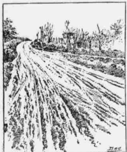
SHOWING HOW GRAVEL IS DEPOSITED AT FOOT OF A HILL WHEN PLACED ON STEEP GRADES.
