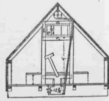
CROSS SECTION OF A SHAPED COLONY HOUSE, SHOWING POSITION OF WINDOW, GASOLINE CAN, PIPE AND HEATER BOX
