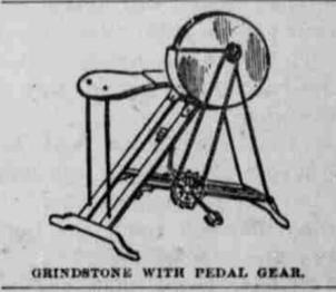
GRINDSTONE WITH PEDAL GEAR.
