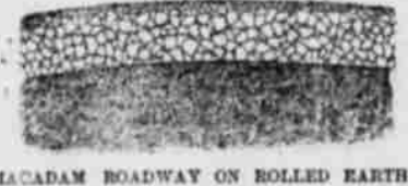
MACADAM ROADWAY ON ROLLED EARTH FOUNDATION.
