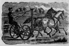
The lightest running Mower made. It is an Iron frame front cut Mower.
