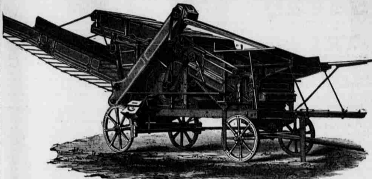
Has Long Straw Bale. Separate Cleaner from Straw. Has long apron and Short Straw Bale. It has the Short quick and Shake on Shoe. Never Clogs in Tar weed or Fern and does not throw grain over. Loss Bells. The city belt passes around the beater and Fan Pulley and is provided with a lighter square gear is substituting for the troublesome iron belt. Creaks less. It is more durable and thrashes faster than any machine in America. If you want to purchase or rent, please write us and we will gladly mail you our catalogue.
