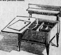
represents the top of the table, open, the body of the table. the space for mixing ingredients. the space for mixing atensils, the space for 25 lbs. meal, the space for 50 lbs. flour, the tray, spices and essences, the kneading board.
