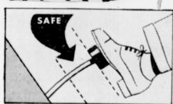
SAFE: Two or more inches clearance between the bottom of your brake pedal and the floorboard normally indicates good brakes . . . which should completely stop your car within 30 feet or less when traveling at 20 miles per hour.
