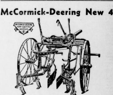
World's Most Popular **Riding Cultivator** SLIGHT pressure on one of the pedals of the A New 4 pivots the wheels and shifts the gangs at
