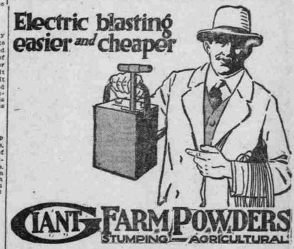
The use of an electric blasting machine results in economy. It reduces the amount of powder required often by 10% to 20%. With it you can shoot several stumps or other blasts at one time. You can fire several lighter shots under a difficult stump or rock with better effect and less trouble than with a single large charge. It is the only reliable means of explodcharges under water.
