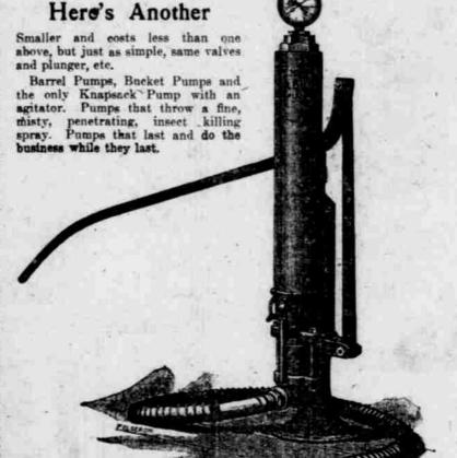
Has solid plunger, long lever, 36-inch air chamber, powerful agitator, most simple, a common wrench is all that's needed to take it apart and set it up. Has two discharge valves, two sprays can be used at once, drains completely.
