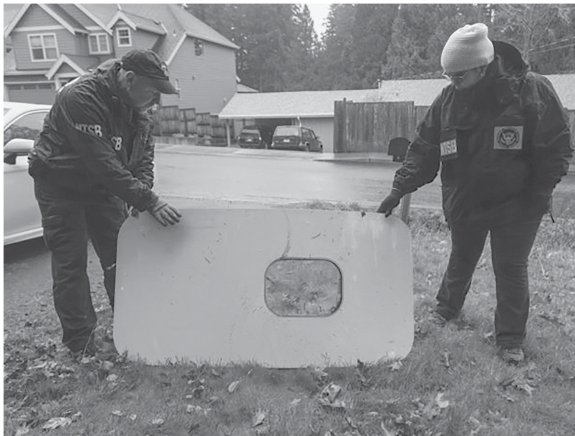
This photo released by the National Transportation Safety Board shows the door plug from Alaska Airlines Flight 1282 on Monday, Jan. 8, 2024, in Portland, Ore. A panel used to plug an area reserved for an exit door on the Boeing 737 Max 9 jetliner blew out Jan. 5, shortly after the flight took off from Portland, forcing the plane to return to Portland International Airport. (National Transportation Safety Board via AP) © Provided by The Associated Press
