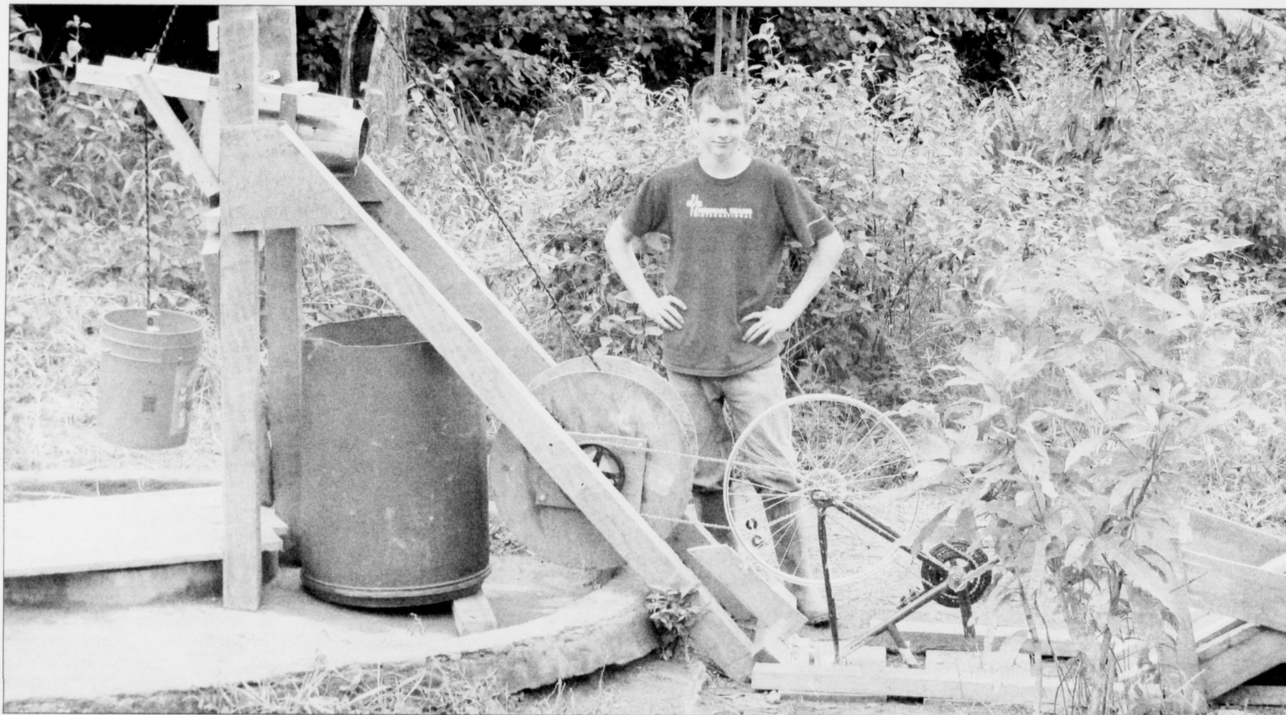
Ben Ulmer, a 2012 graduate of Oregon Episcopal School is shown in Liberia with a bicycle-powered pump that he and other students designed and that he field-tested in the west African country.
