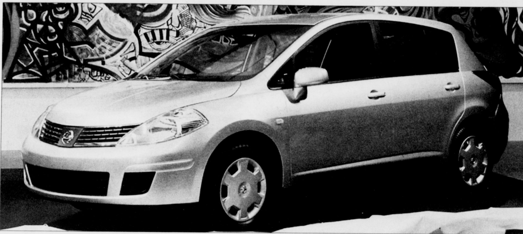
Tested Vehicle Information: 1.8L 4 Cylinder engine; Xtronic CVT transmission; 28 City MPG, 34 Highway MPG; MRSP $16,900 Tested Vehicle MSRP $18,405.
