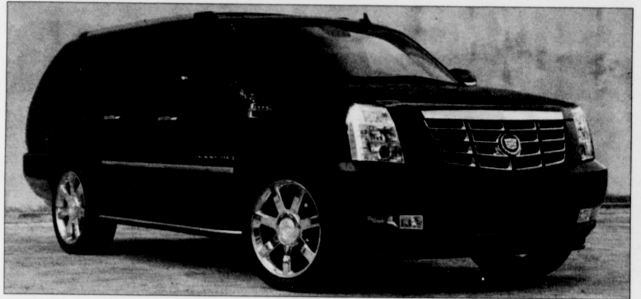
Tested Vehicle Information: Vortec 6.2L V8 SFI, 403 HP with Flex-Fuel Capability and Active Fuel Management; 6-Speed Heavy Duty Automatic; 13 City MPG, 18 Highway MPG; MSRP $87,345, Tested MSRP $88,295.
