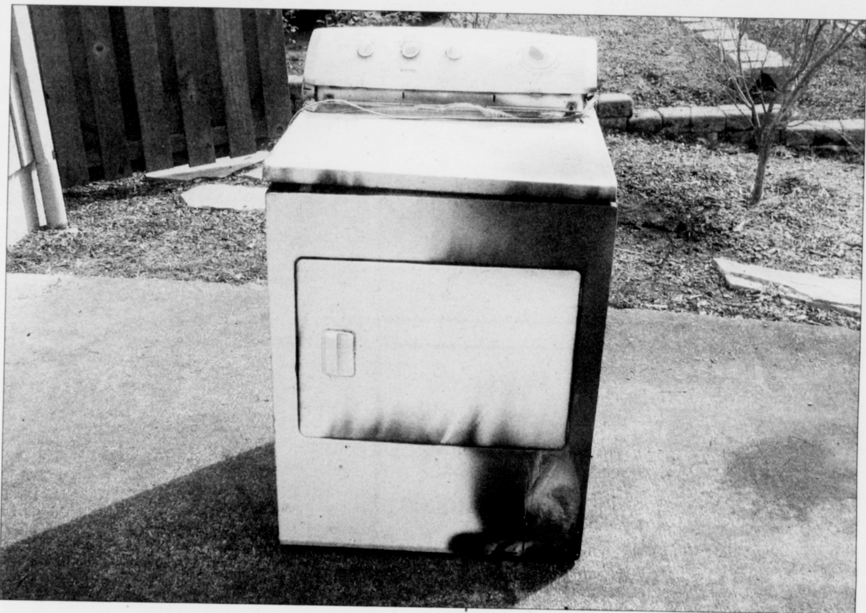
Tualatin Valley and Fire Rescue provided this picture of a clothes dryer charred from a fire that started because of improper maintenance and venting caused by the build-up of lint.
