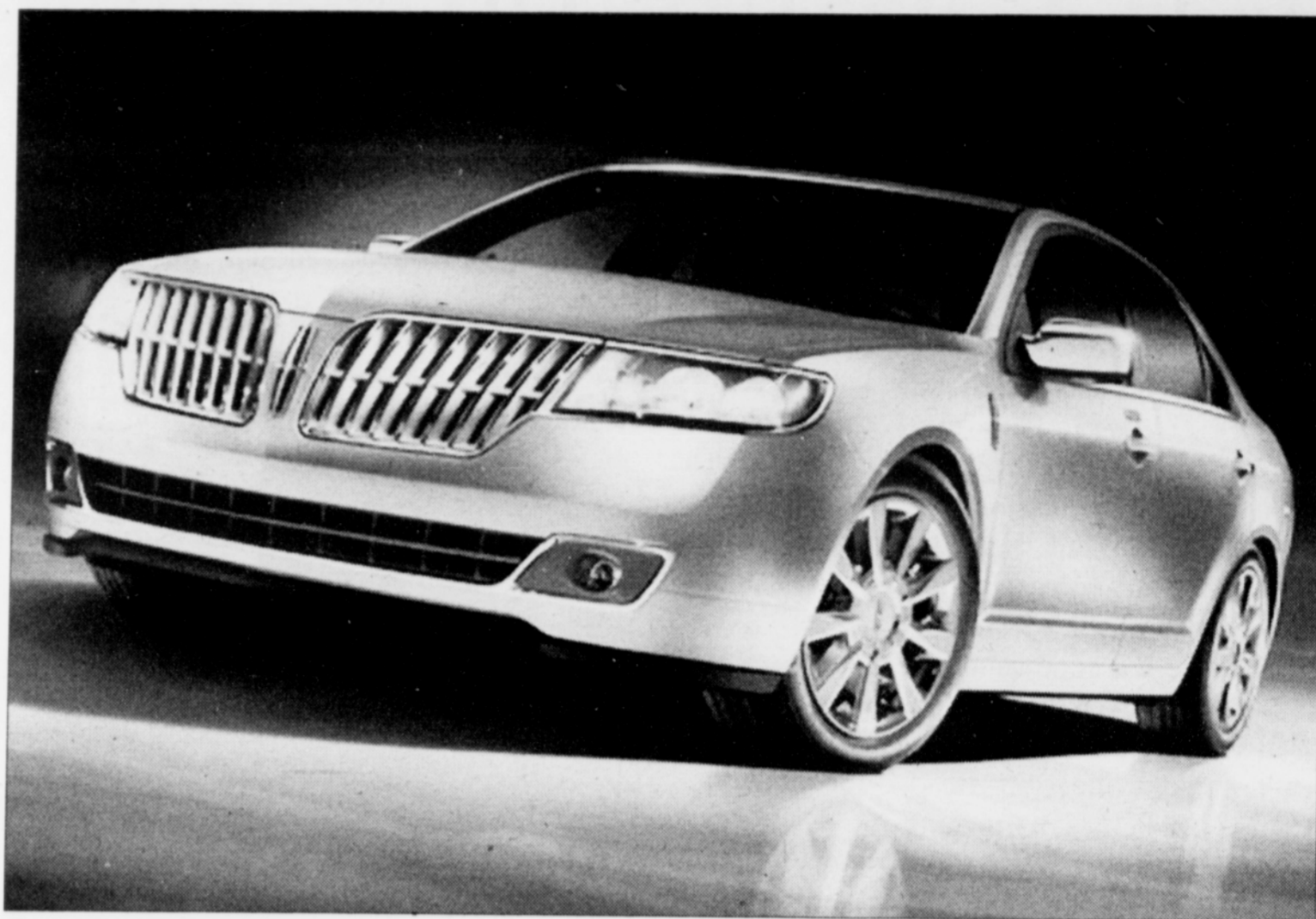
Tested Vehicle Information: 3.5L 24 V6 Duratec engine; 6-speed selectshift automatic transmission; 17 city mpg, 24 highway mpg; MSRP $36,005 Test Vehicle MSRP $43,245.
