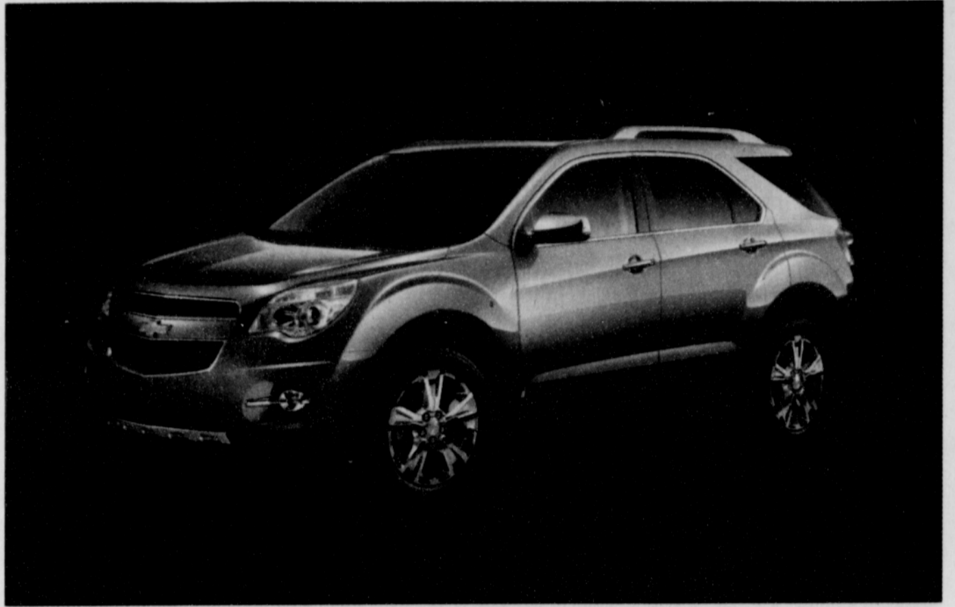
Vehicle Specifications: 2.4L 4 cyl, DOHC SIDI; 6 speed automatic transmission; 22 city MPG, 32 Highway MPG; MSRP $28,045 Test vehicle price $32,230.
