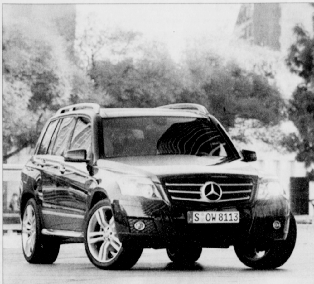
Vehicle Specifications: 3.5L V6 24-Valve gasoline engine; Seven speed driver adaptive automatic transmission; 15 city mpg, 20 highway mpg; MSRP $45,685.
