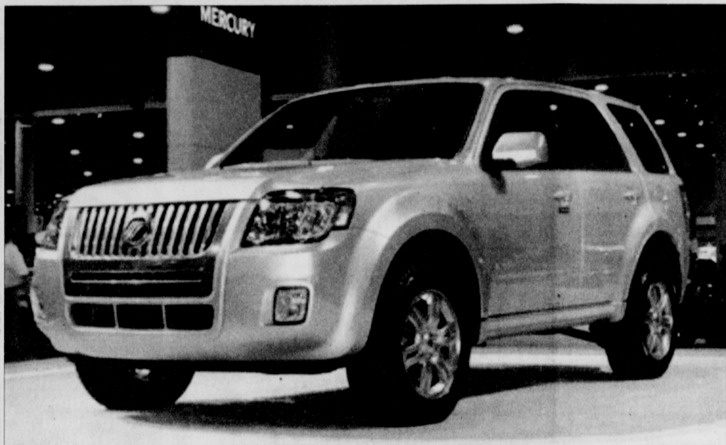
Specifications: 3.0-Liter, 240-hp @ 223 lb-ft. torque, DOHC 24-valve V-6 engine; 6-Speed automatic transmission; 17-City, 24-Highway MPG; $32,795. MSRP
