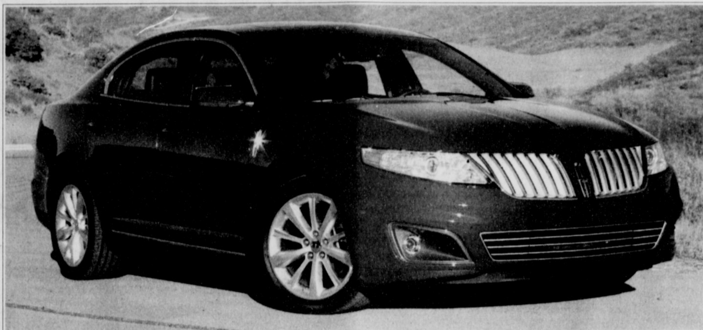
Specifications: 3.7-Liter, V-6, 24-valve, 273-hp @ 270 lb-ft. torque engine; 6-Speed automatic transmission w/ select shift; 17-City 24-Highway; $44,570. MSRP
