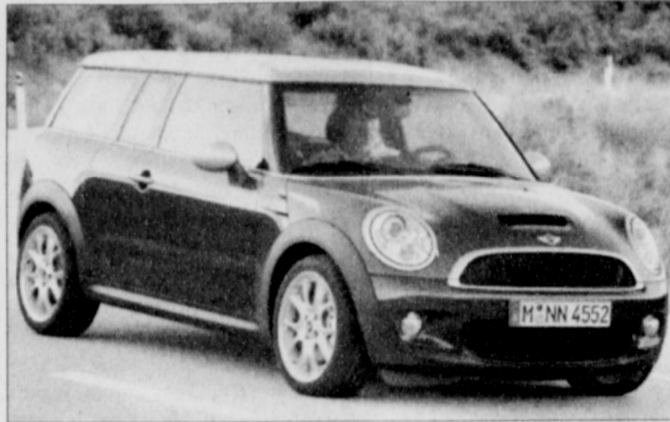
Specifications: Dual overhead cam 1.5-liter inline 4-cylinder engine; 6-speed manual transmission; 28-City 37-Highway MPG; $28,700, MSRP
