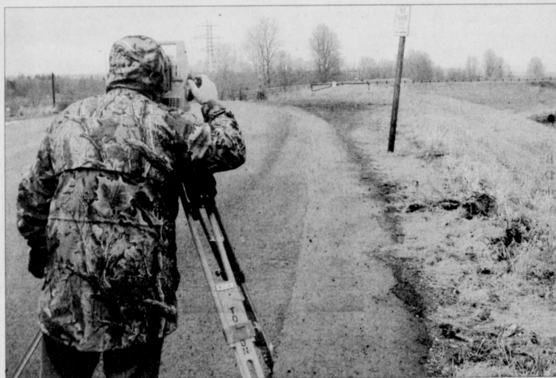
The U.S. Army Corps of Engineers surveys a levee near the Columbia River in early 2007. Data from these surveys help owners determine a levee's level of flood protection. Trees along some of the levees present an increased risk because they were not designed for this type of vegetation.
