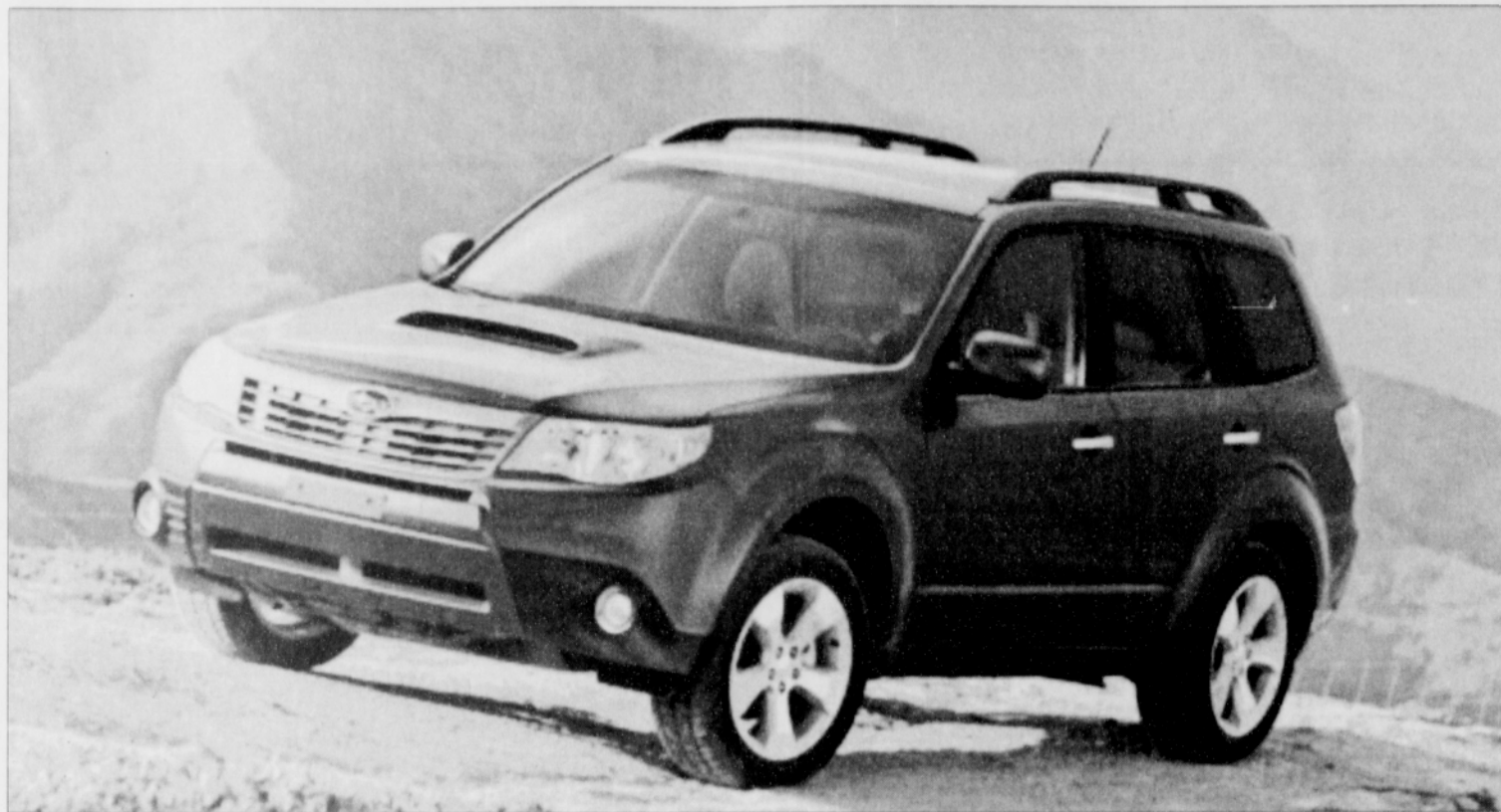
Specifications: 2.5-Liter 4-cylinder 224-hp @ 226 lb-ft. torque turbocharged engine; 4-speed automatic w/manual-shift mode transmission; AWD; 19-City 24-Highway MPG; $30,660. MSRP
