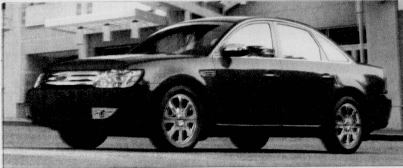
Specifications: 3.5-Liter, 24-valve 263-hp @ 249 lb-ft. torque, V-6 Duratec engine; 6-speed automatic transmission; 17-City, 24-Highway MPG; $ 33,600. MSRP
